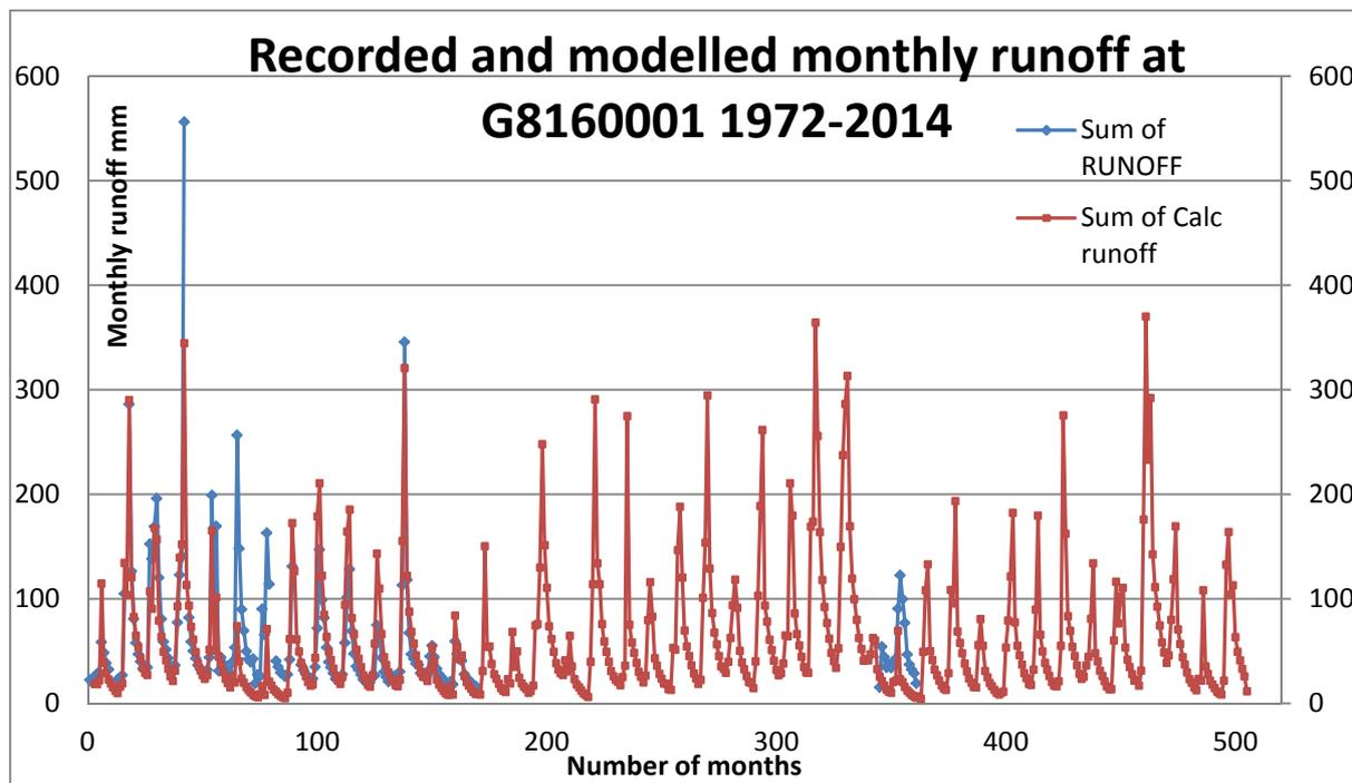
Figure 5-17: Recorded and AWBM modelled monthly runoff at G8160001
