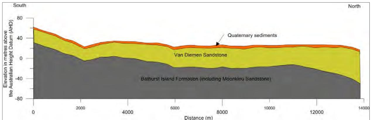
Figure 2-2: South to north cross-section of sub-surface geology (Hughes 1976)
