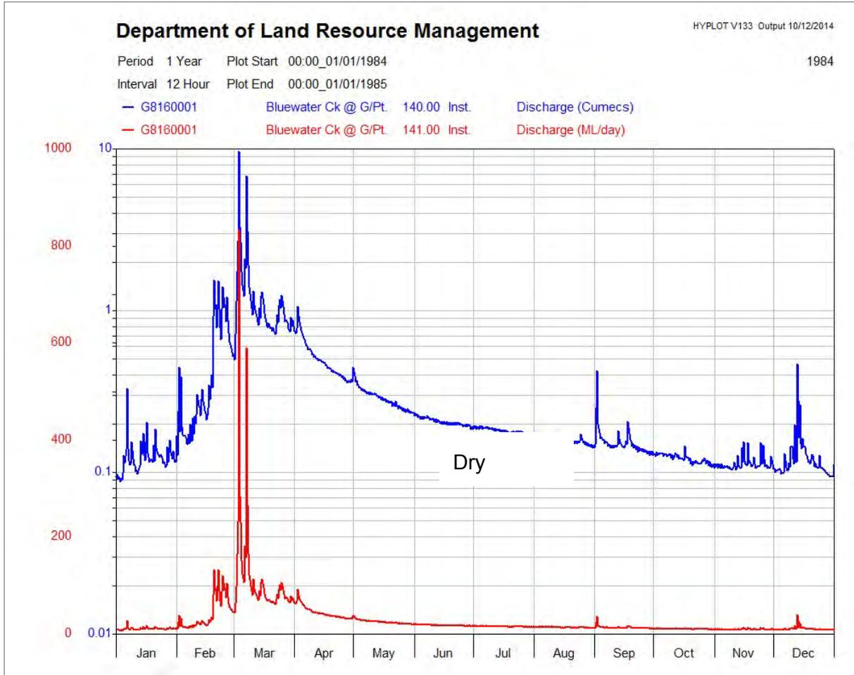
Figure 5-5: Discharge hydrograph for Bluewater Creek, Site G8160001 for 1984
