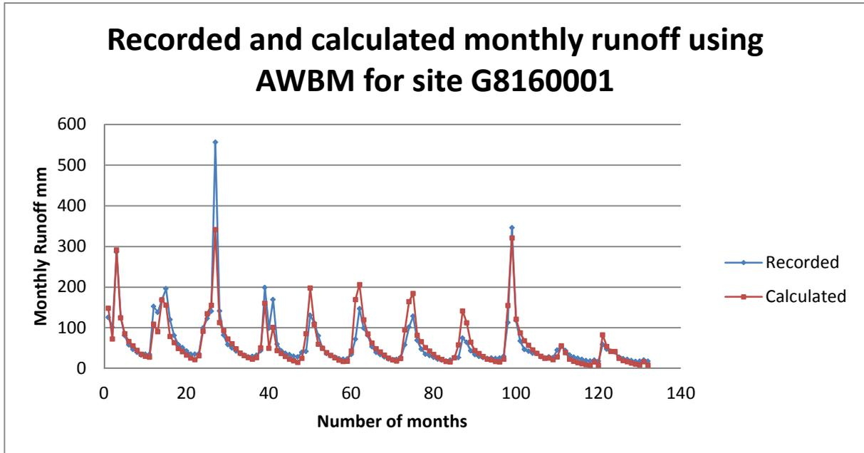
Figure 5-16: Recorded and AWBM modelled monthly runoff at G8160001
