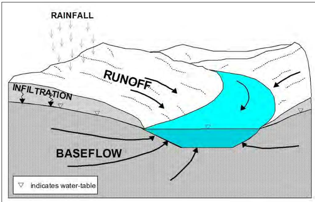
Figure 5-4: Runoff and baseflow components of surface water
