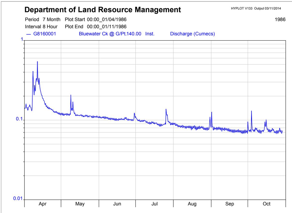
Figure 5-15: Effect of small rain events on baseflow at G8160001
