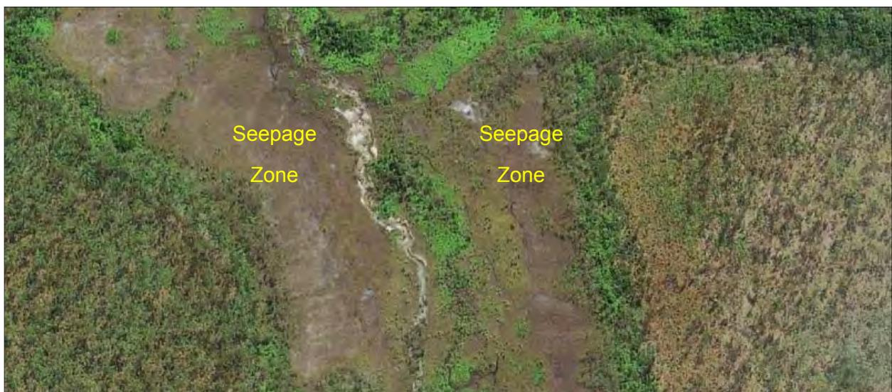
Figure 5-8: Satellite imagery showing seepage zones on Bullabolla Creek
