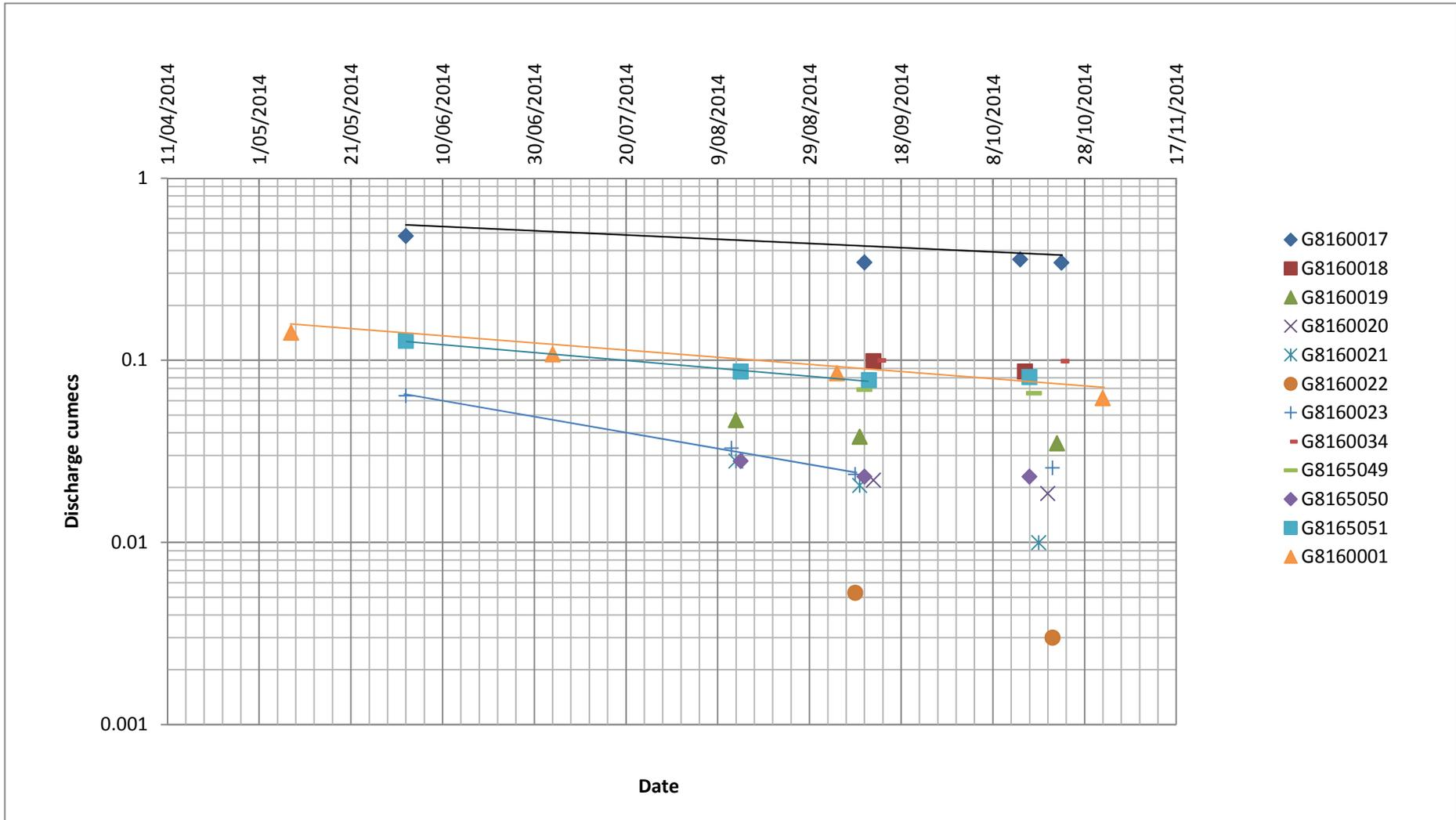
Figure 5-14: Flow gauging undertaken in 2014. 1985 flow data at G8160001 is also plotted.
