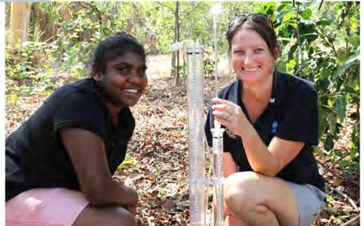
Jessica Stassi and CSIRO's Jodie Hayward using an infiltrometer to measure how much water soaks into Top End soils (rather than running off) during the first storms of the wet season.
