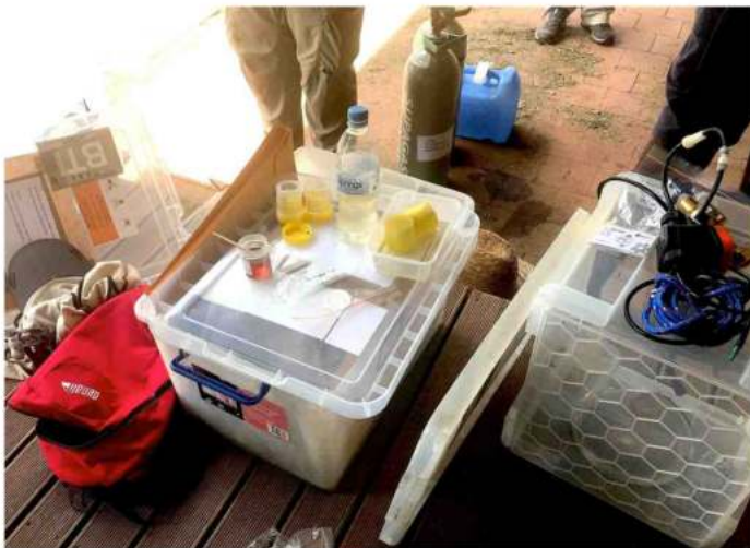
Preparing the Honey coated FTA card used in the SMACK traps
